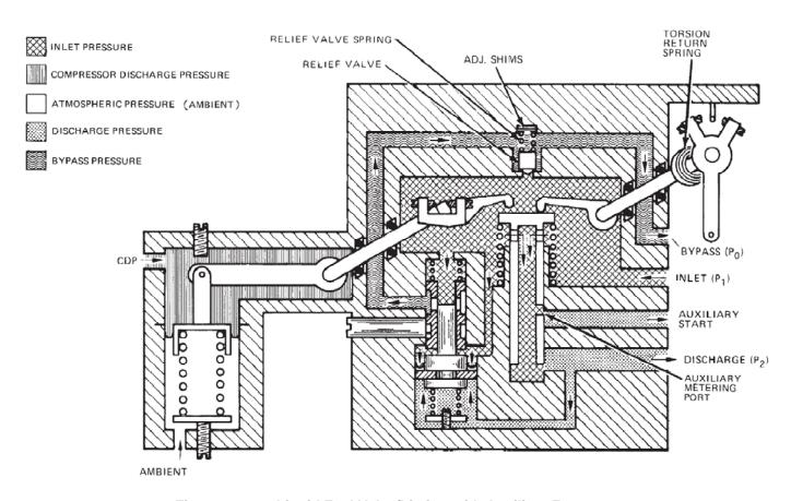
Figure 3. 1907 Liquid Fuel Valve/Limiter with Auxiliary Features
