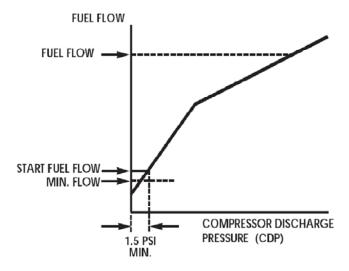
Figure 1. Fuel Flow vs Compressor Discharge Pressure (CDP)
