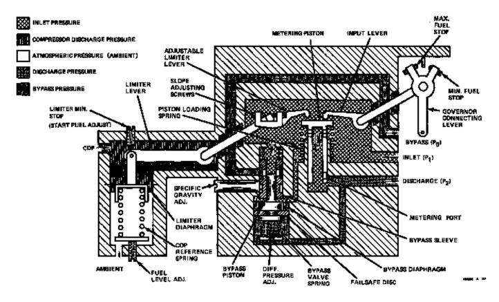
Figure 2. 1907 Liquid Fuel Valve/Limiter
